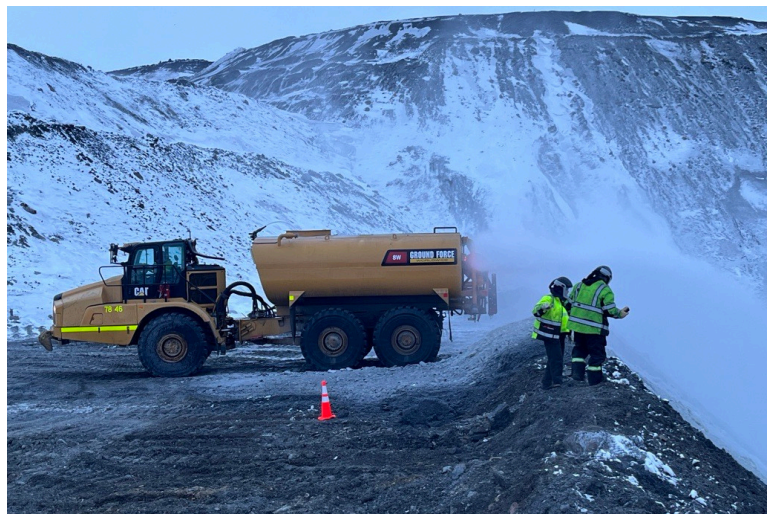
Mine Ops personnel apply water to reactive waste materials in MPD4.
